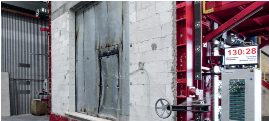
Fire Test, view after 130 minutes
