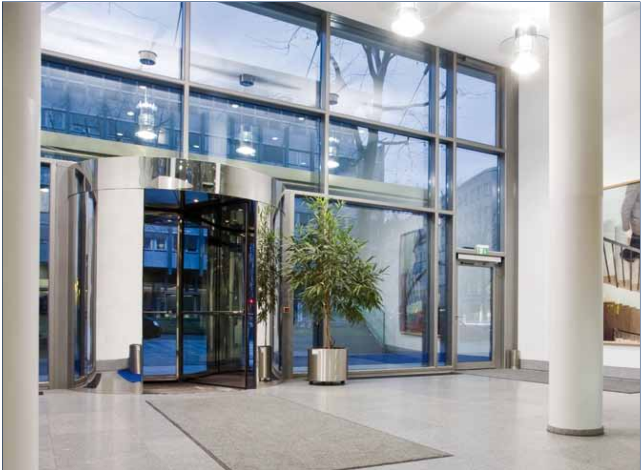
Deutsche Bank, Stuttgart - Fully-automatic GEZE revolving doors with 3 leaves and drum walls of sheet metal panels
