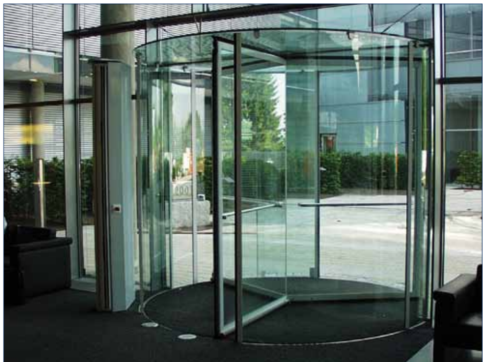
CSC Plönzke, Wiesbaden Fully-automatic GEZE revolving door with 3 leaves and outside night locking mechanism and movement detectors in the floor
