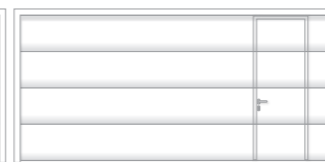
Asymmetrical position on garage doors measuring BRB 2000 - 3500 mm - left or right of centre
