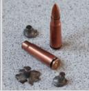
Calibre 7.62 x 39 Bullet weight 8.0 g Impact at 720 m/s Impact force of pointed bullet with iron core 2074 J
