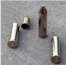
Calibre .357 Magnum Bullet weight 10.2 g Impact at 430 m/s Impact force of coned bullet 943 J
