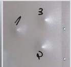
The associated deformation of steel armour. The projectiles were stopped effectively.
